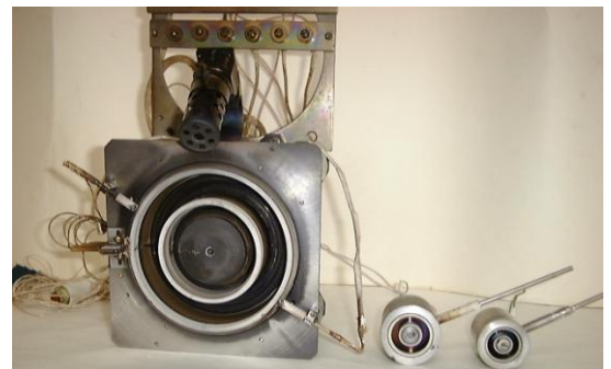
Figure 3 – Laboratory Model of the SPT-100 (in the Left) and SPT-25, SPT-20 (in the Right)
