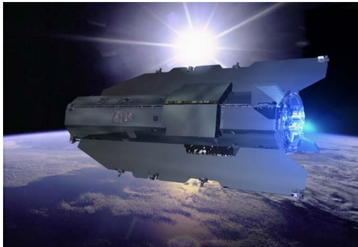
Figure 1 - ESA's low-orbit scientific satellite GOCE with ion thrusters for air drag compensation
