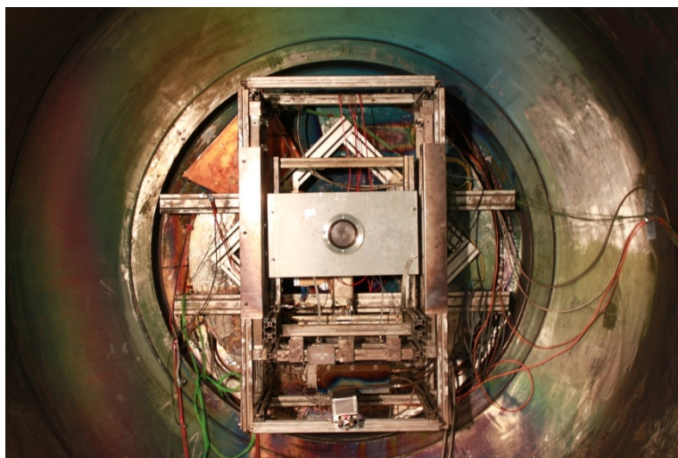
Figure 5 - RAM RIT-10 thruster mounted at the thrust balance of the 30 m 3 vacuum test facility JUMBO at Giessen University
